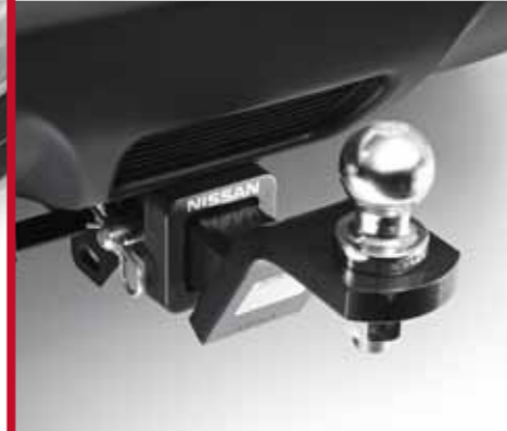
Towbar & Towball Maximum braked capacity of 1500kg (CVT Petrol)
