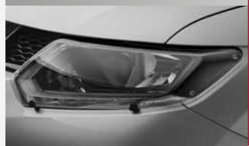
Headlamp Protectors Helps protect headlamp from the impact of stones and other road debris
